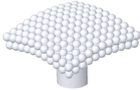
Fig. 6: Simulated 3D deformed particle model of a rubber sheet after impacting a cylinder
